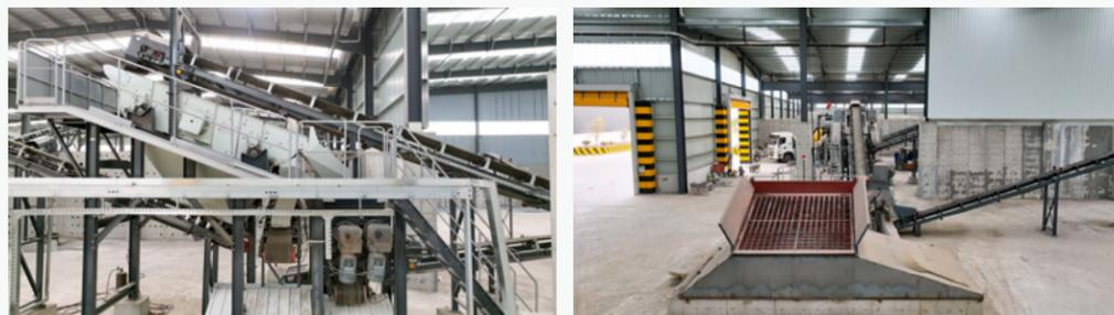
Asphalt Milling Material Crushing and Screening Equipment
