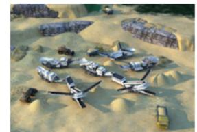
Mobile Demolition Waste Processing Line
