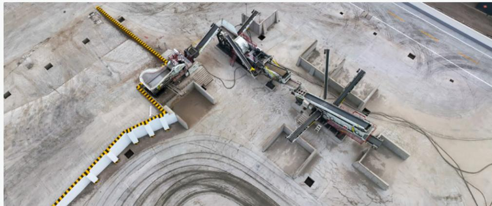
Frame-type Mobile Crushing and Screening Production Line
