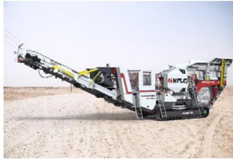
The E-Series Electric-Driven Mobile Crusher
