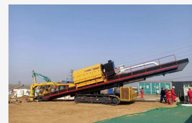
XTC150G, the world's first diesel-electric dual-power double-wheel milling machine
