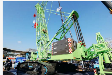
XLC450 DP Crawler Crane, an industry-exclusive 450-ton dual-power (DP) crawler crane
