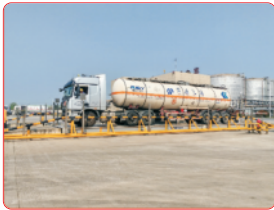
Unmanned Weighbridge System with Automatic Identification
