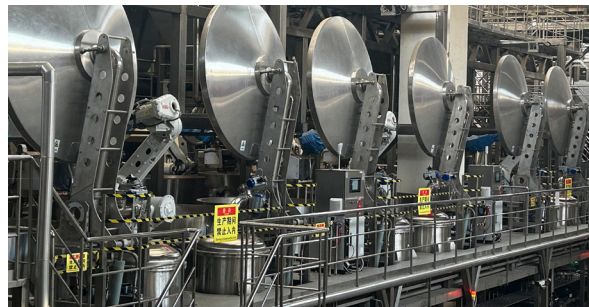
Automated Operating Process of Steaming Fermented Materials at the Gujing Intelligent Industrial Park
