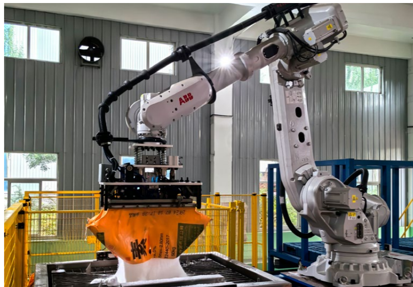
❖ Urea feeding robot realizes intelligent SCR catalyst flow
