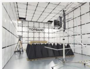
3m method anechoic test chamber facility (radiated immunity)
