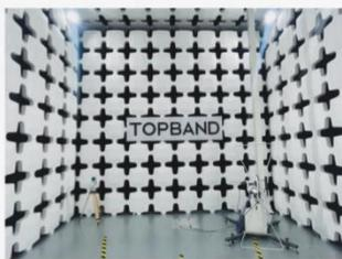
3m compliant semi-anechoic test chamber facility (radiation emission)
