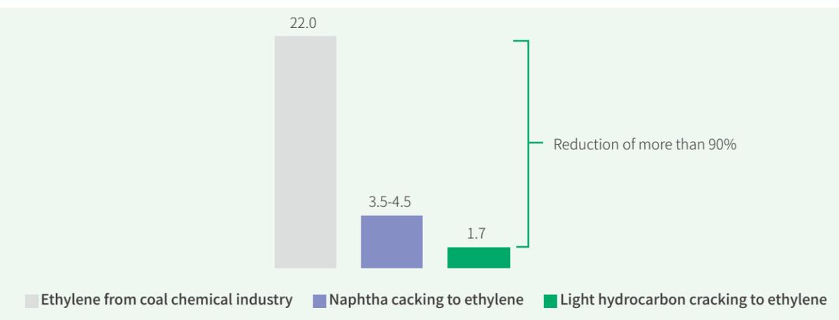
Water consumption of light hydrocarbon cracking compared to other processes for ethylene production (metric tonne of water/metric tonne of ethylene)
