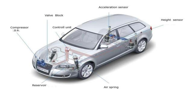
Compare to coil spring suspension, air suspension system has the advantage that the Spring stiffness can be adjusted according to different usage scenario. Base on the different road conditions and the input from the height and acceleration sensor, the ECU of ECAS system will identify the vehicle height change, the air height of air spring can be adjusted through the control the air compressor and valve block to realize the lift or lowering of the vehicle body.
