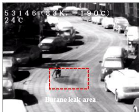
Gas Leak Detection (50 meters away, butane) Result
