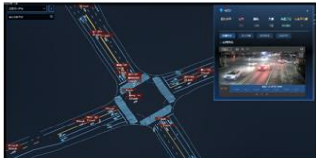
Interface of traffic projection software: distribution of vehicles at intersections (with vehicle speed information)
