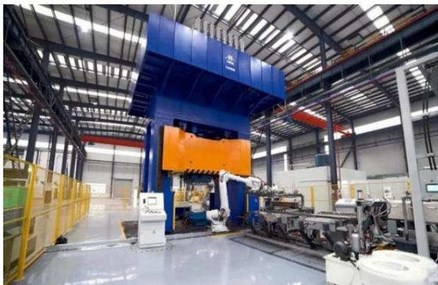
LFT-D 液压机生产线
