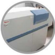
直读光谱仪 Direct Reading Spectrometer 金属成分分析 To test composition of alloys
