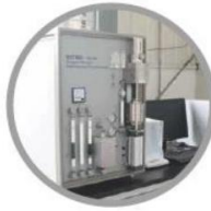
氧分析仪 Oxygen Tester 铜及铜合金中的氧元素检测 To detect oxygen elements of copper and copper alloy
