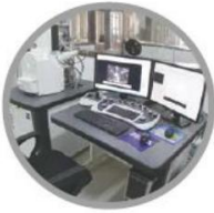
能谱分析扫描电子显微镜 SEM(Scanning electronic microscope with energy spectrum) 微观形貌观察, 微区化学成分定量分析 To observe micro-morphology, and make chemical composition quantitative analysis in small area
