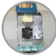
原子吸收光谱仪 Atomic Absorption Spectrometer 原料微量元素检测 To detect trace elements of raw materials
