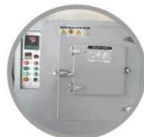
耐高温测试仪 High Temperature Resistance Performance Tester 测试耐高温性能 To test high temperature resistance performance
