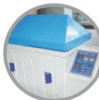
盐雾性测试仪 Salt Spray Tester 耐腐蚀性测试 To test corrosion resistance performance
