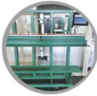
LED 数字测微仪 LED Digital Micrometer 金属带材宽度和曲率测试 To measure strip width and camber
