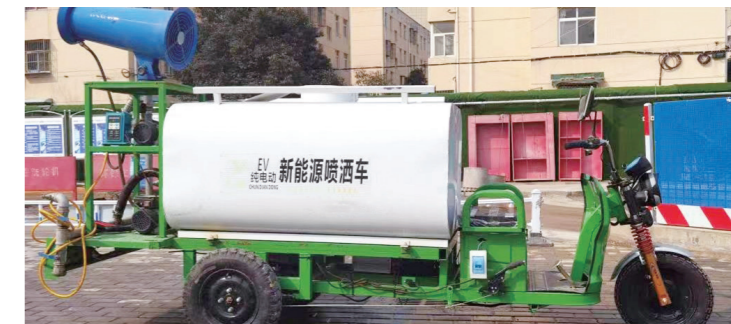
通号工程局集团使用小型新能源喷洒车，减少扬尘污染 Engineering Group adopted small NEV spraying vehicles to reduce dust pollutions
